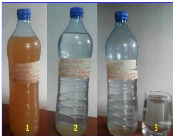
SaferEx - Multi-action Water Purifier used in treatment and recovery of safe water from muddy, heavy metal and pathogen infested raw borehole water from Okposi Town, Oshosara L.G.A, Eboymi State, Nigeria (in situ treatment). 1. Raw and heavily contaminated borehole water from Okposi town, Eboymi State, Nigeria. 2. Raw water after treatment with SaferEx Multi-action Water Purifier with sediments (1-2hr) 3. Purified water in a cup after SaferEx treatment and decantation (>80% of safe water recovered)
