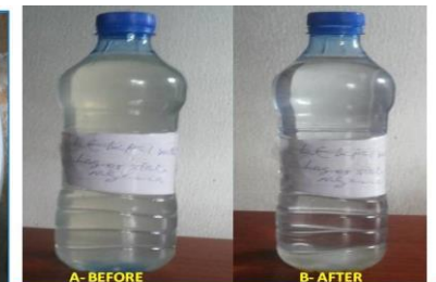
SaferEx in situ treatment of household borehole water from LEKKI, Lagos State, Nigeria analyzed and contains pathogens, metals and salts. A -Before treatment with SaferEx B -After treatment with SaferEx with sediments; rid of pathogens, salts and unwanted metals prior to filtration (after <45 minutes).
