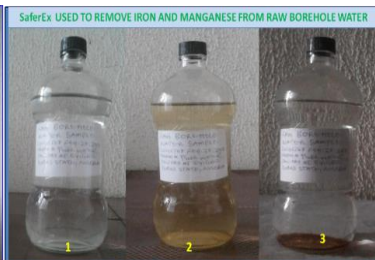
SaferEx USED TO REMOVE IRON AND MANGANESE FROM RAW BOREHOLE WATER Raw borehole water at Oyiabo town, Rivers State, Nigeria analyzed to contain high Iron and Manganese but remains clear in appearance. (Collected from a water packaging factory). 1. Raw borehole water analyzed to contain Iron and Manganese but clear in appearance. 2. Raw borehole water after adding 5ml SaferEx -Multi-action Water Purifier (after <10 minutes). 3. Borehole water with Iron and Manganese sedimented after treatment with SaferEx to remove Iron and Manganese.
